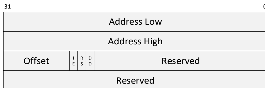
Figure 12-5. Receive Descriptor Structure (Posted by Host)
