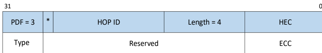
Figure 10-10. ACK Packet Format
